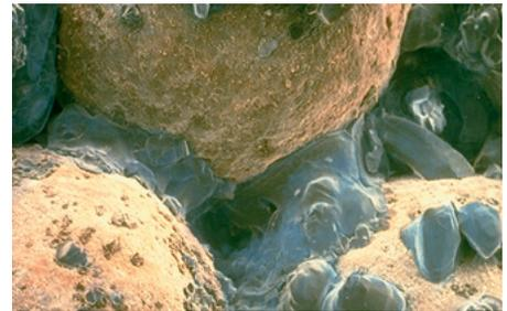
Crystal bridges between fertilizer particles cause caking
